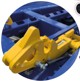
Height of the tow bar is adjustable
